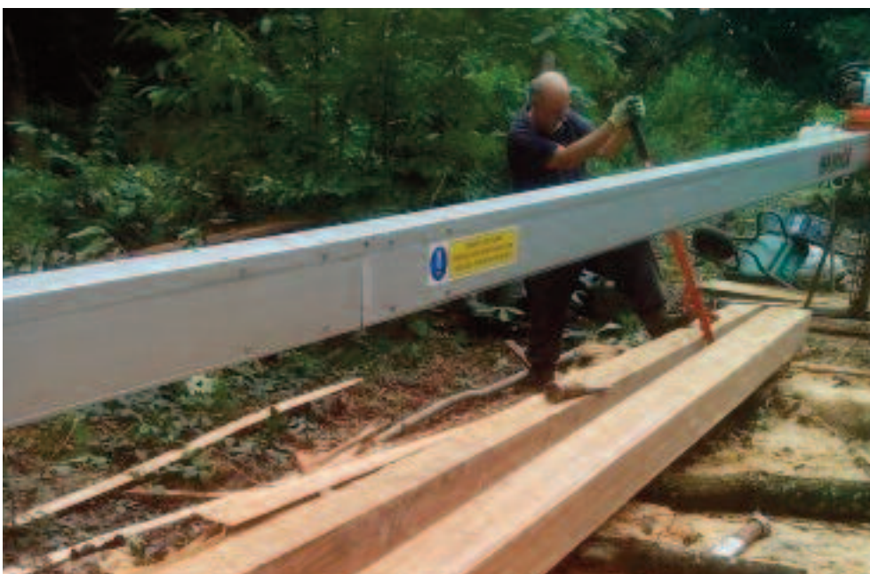
Swing arm milling an 8"x8 beam.
