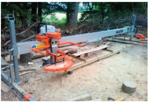
purchased a swing arm portable mill manufactured in New Zealand by Turbosawmill.
