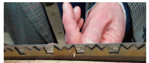
Get a feeler gauge between the straight-edge and one tooth.
