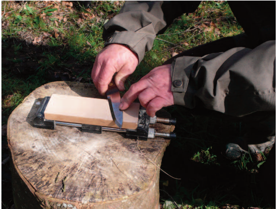
Sharpening a knife on a whetstone
