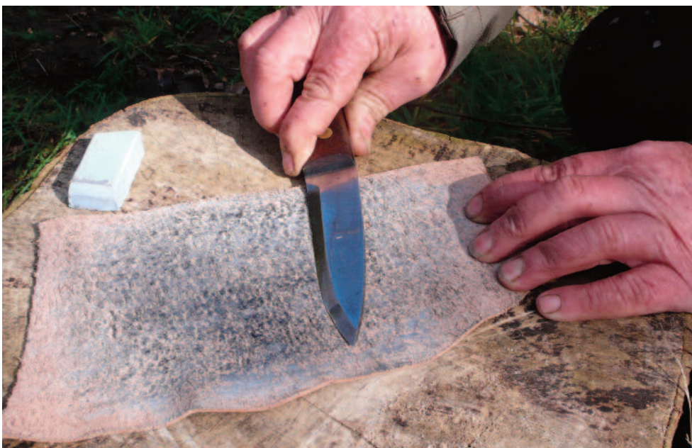
Polishing a blade using starkie blue
