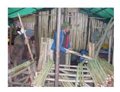
the woods. A notched jig enables him to cut to the desired lengths at a glance and single-handed.
